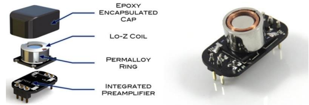
Figure 14. Nu Capsule self-contained active pickup
